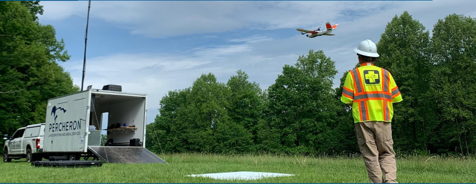
Percheron partnered with TC Energy to execute an exploratory project investigating the process of obtaining a Beyond Visual Line of Sight (BVLOS) waiver from the FAA, and the viability of executing BVLOS UAS flights in a real-world scenario along a pre-selected Right of Way in the Northeast.
